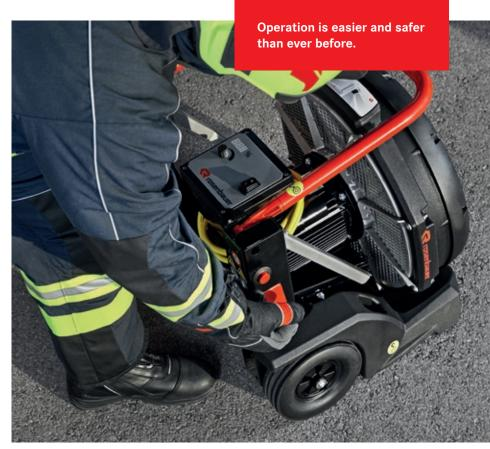
The E and V models can be brought into the first attack position (+20°) with a single movement.
